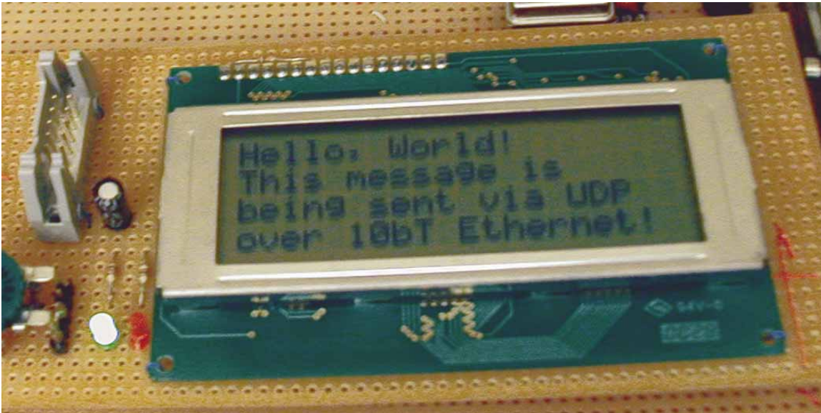
Figure 3: The device receives the UDP message, and displays the contents as ASCII
